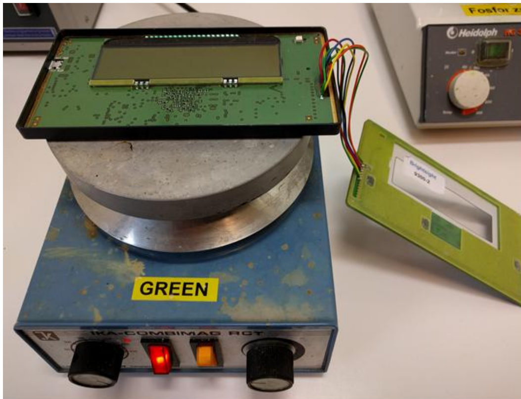
Figure 11: Setup for heating experiments: demonstrator on top of hot plate.
