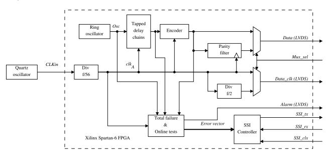
Figure 2.5: Block diagram of the DC-TRNG design
