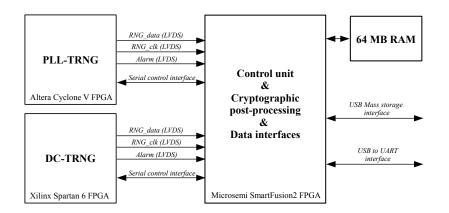
Figure 2.1: Functional block diagram of the HECTOR Demonstrator 1 platform
