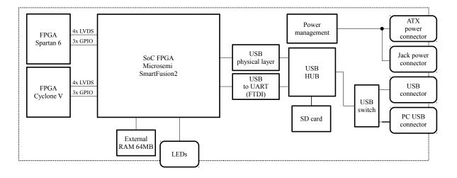
Figure 2.2: Block diagram of the HECTOR Demonstrator 1 hardware
