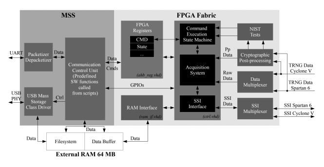
Figure 2.7: Block diagram of hardware means in Demonstrator 1 SoC
