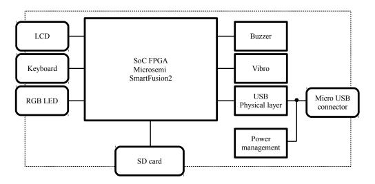
Figure 3.2: Demonstrator hardware platform.
