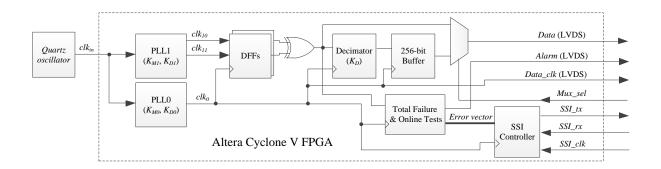
Figure 2.4: Block diagram of the PLL-TRNG core implemented in Altera Cyclone V FPGA as a part of HECTOR Demonstrator 1
