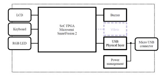
Figure 4.2: Demonstrator 3 hardware platform.
