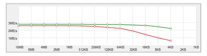
Figure 3.6: Data transfer rate. Reading in green, writing in red.
