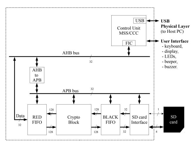
Figure 3.3: FPGA top architecture.
