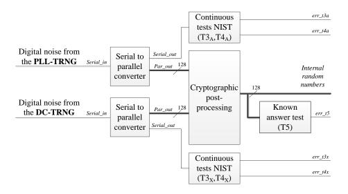
Figure 2.6: Block diagram of hardware in the Demonstrator 1 control device
