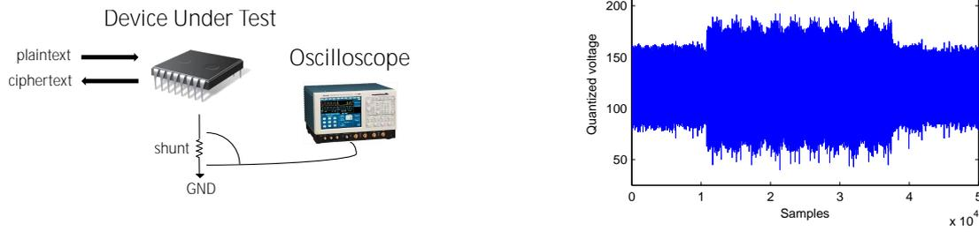
Figure 5.1: Experimental setup to measure power consumption of a device (left). Exemplary power measurement from an AES-128 execution on an embedded processor (right).
