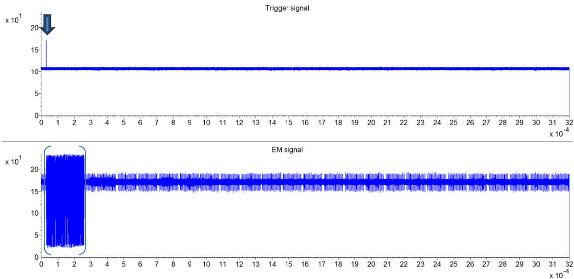
Figure 24: Trigger signal and an example of the interesting pattern (marked by the brackets) observed afterwards. The arrow indicates the start of the statistical test procedure.
