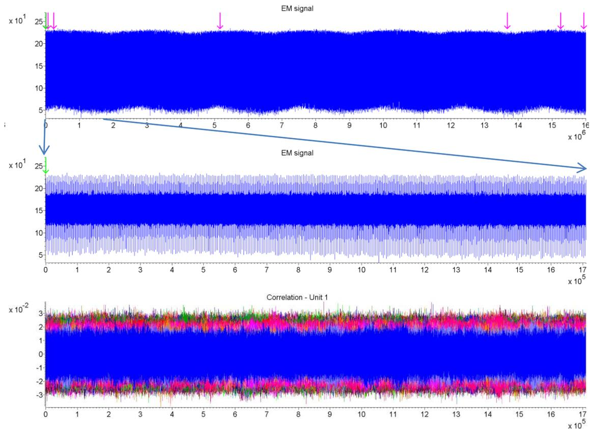
Figure 51: EM signal with arrows indicating the alignment locations (1<sup>st</sup>). A zoomed in view of the first alignment location indicated by the green arrow (2<sup>nd</sup>) and the correlation result using the traces aligned there (3<sup>rd</sup>).
