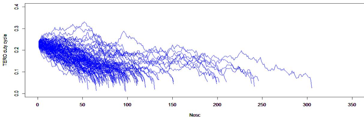
Figure 15: TERO output duty cycle evolution with jitter noise and voltage variation
