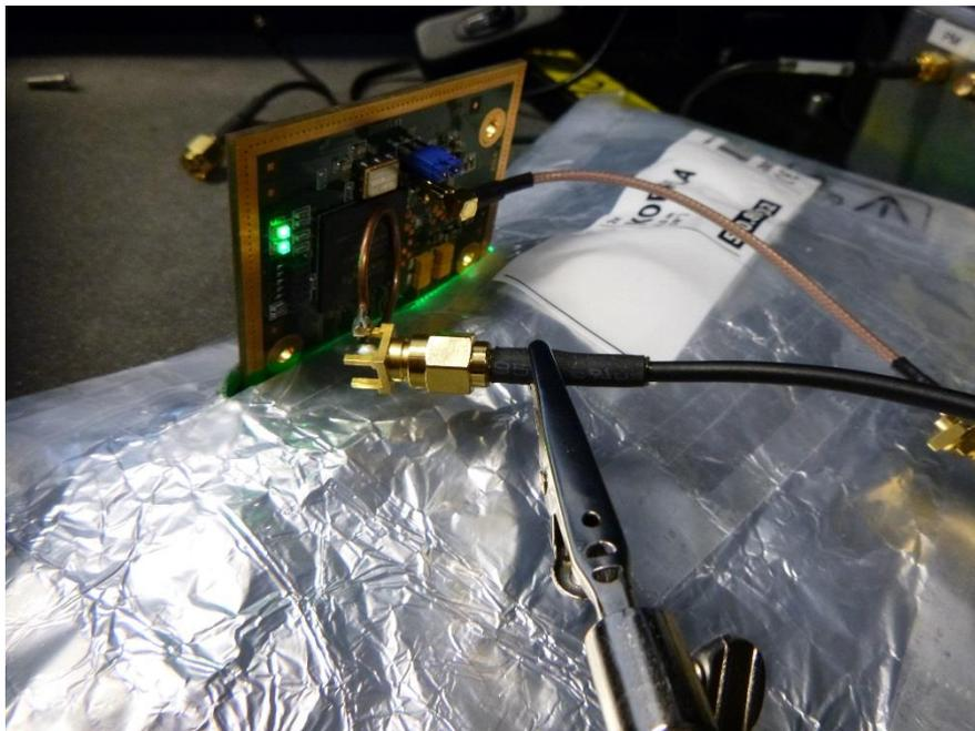
Figure 25: Final coil position for the measurement of configuration #6.
