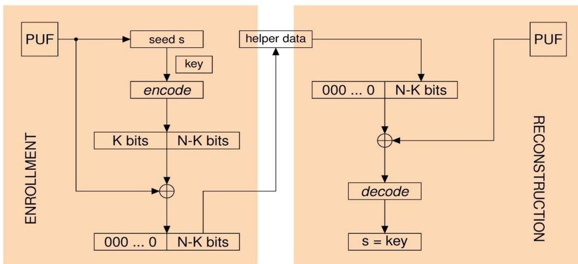
Figure 74: Fuzzy extractor based on codes with systematic encoding (Kang's scheme [2])
