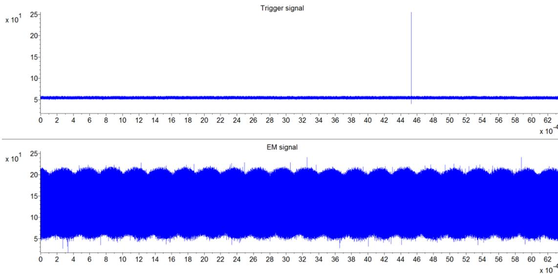
Figure 36: The raw EM signal and the trigger signal. No variation of the EM signal can be seen when the trigger is generated.
