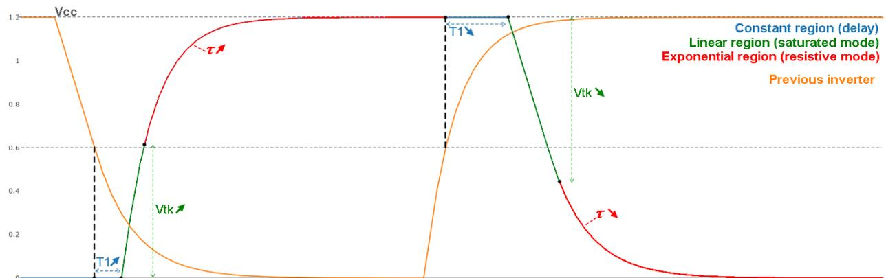
Figure 7: Inverter model
