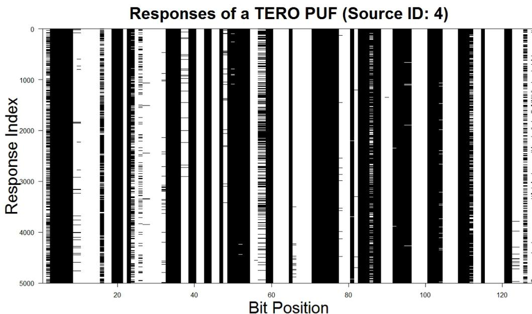
Figure 16: Responses of a TERO PUF with dark bits
