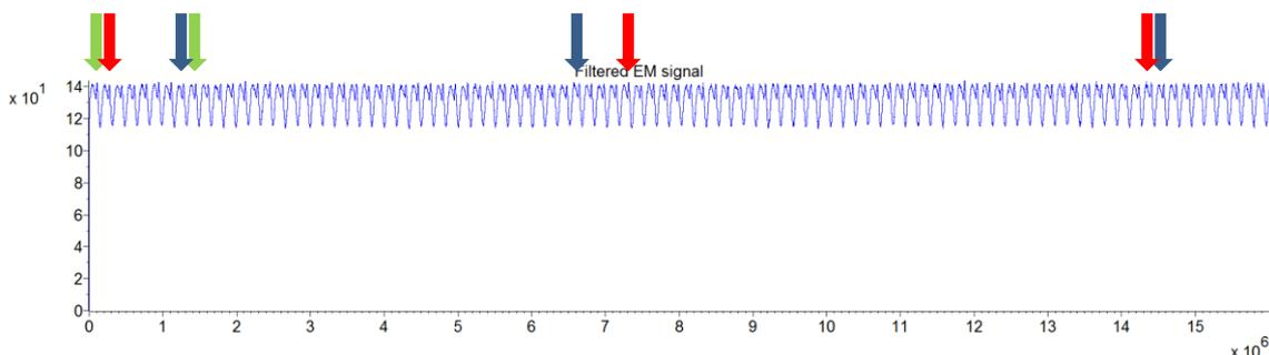
Figure 39: A time-filtered trace. The red and blue arrows indicate the different points of alignment with the two different alignments just in the beginning. The green arrows indicate points which were used for alignment in both cases.
