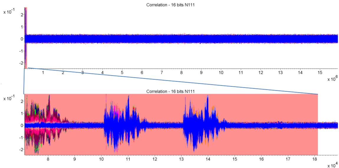
Figure 31: Correlation results for the first 16 bits of the  $N_{111}$  data on the converted traces.
