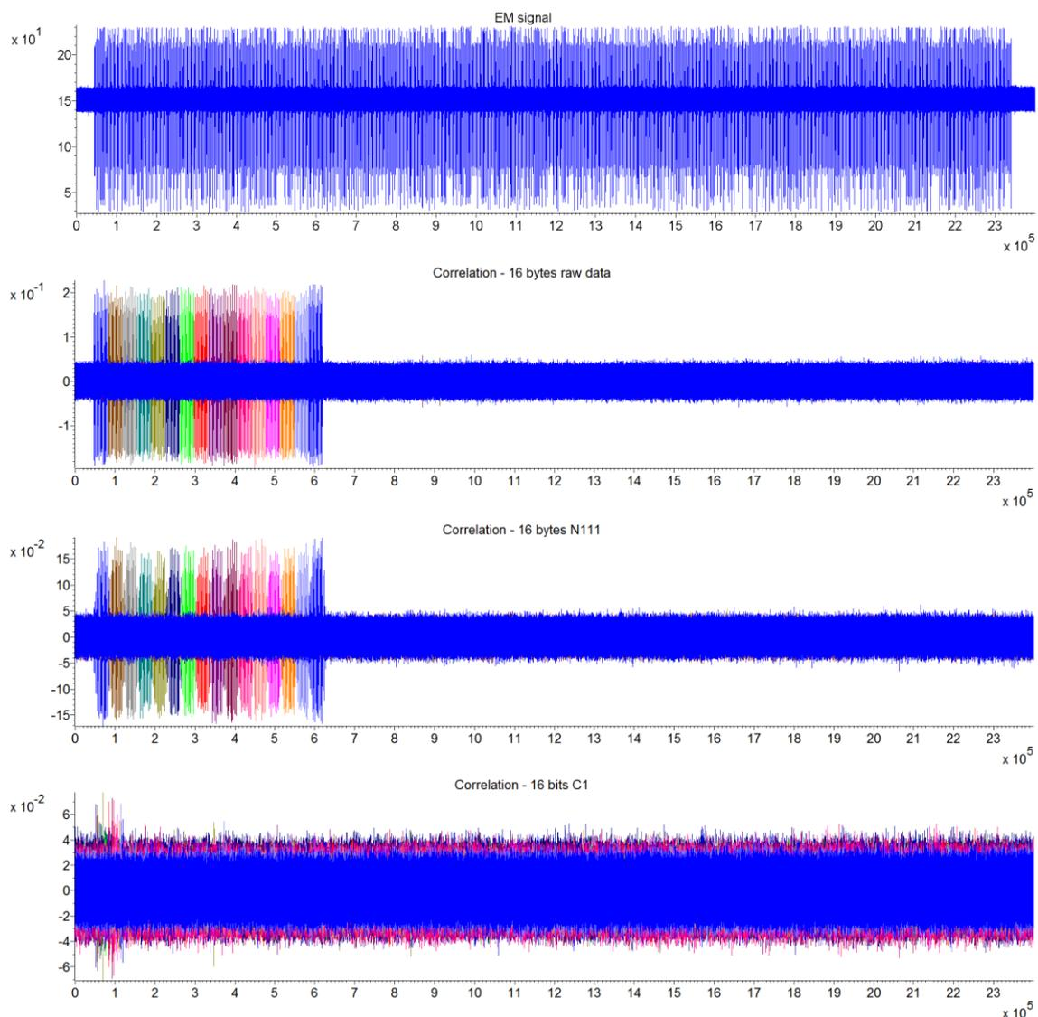
Figure 27: An example EM trace of the first measured set can be seen in the top. The three graphs in the bottom show the correlation results with the raw random data and the data of the statistical tests.
