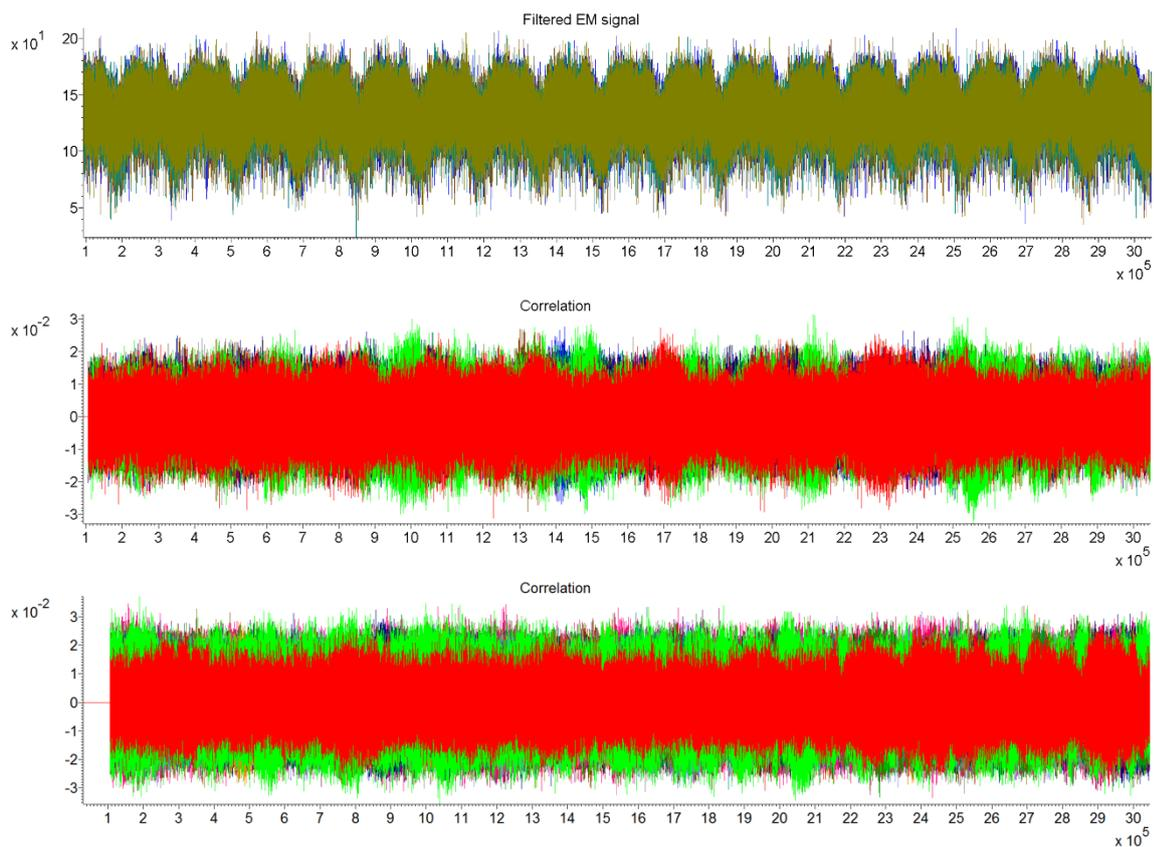
Figure 48: The investigated part of the aligned traces can be seen in the top, the correlation traces of the first eight bytes (middle) and of the first 64 bits (bottom).
