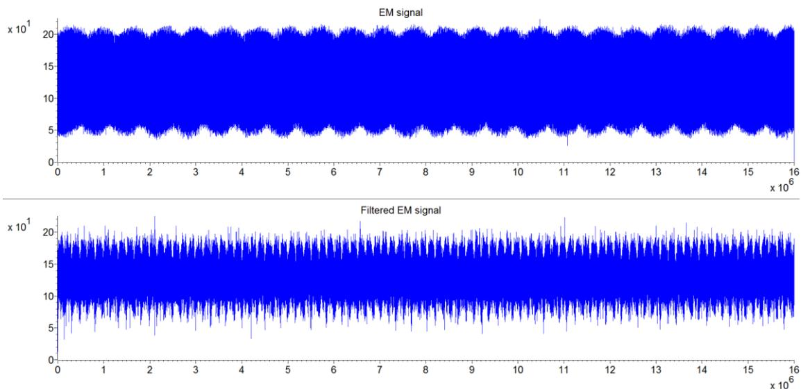
Figure 37: Raw and filtered EM trace of the GET\_CNT measurement
