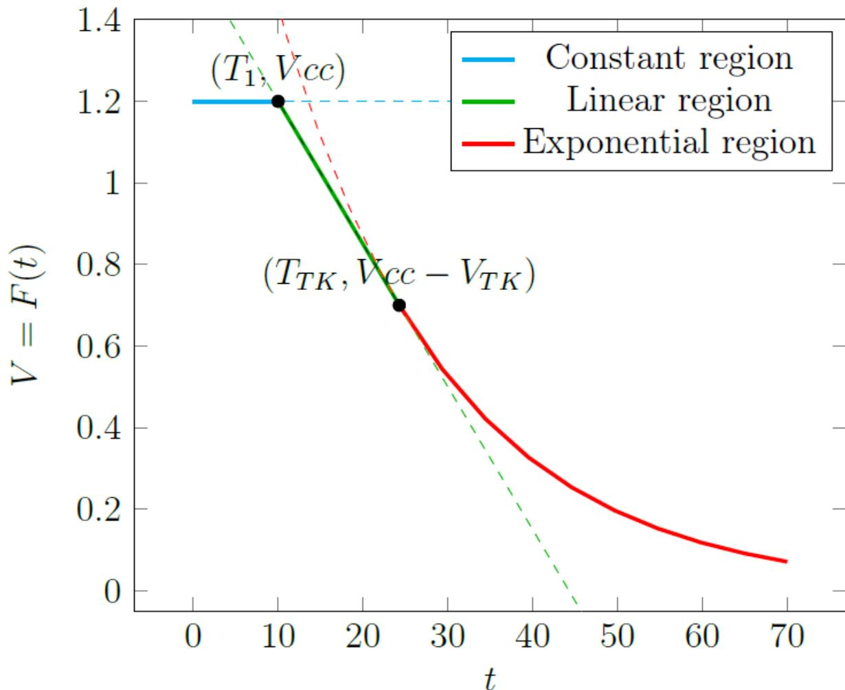
Figure 8: Inverter falling edge model
