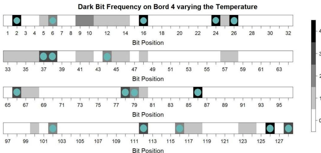
Figure 22: Frequency of being a dark bit at four temperatures on board 4. Blue bits would be thrown away at 25° C as basis.
