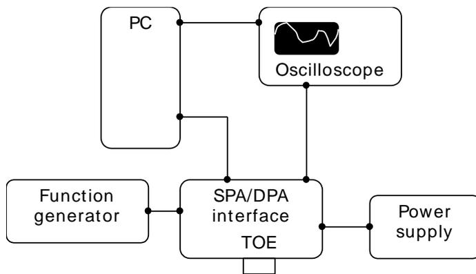
Figure 67: Schematic representation of the set-up (non-contactless).
