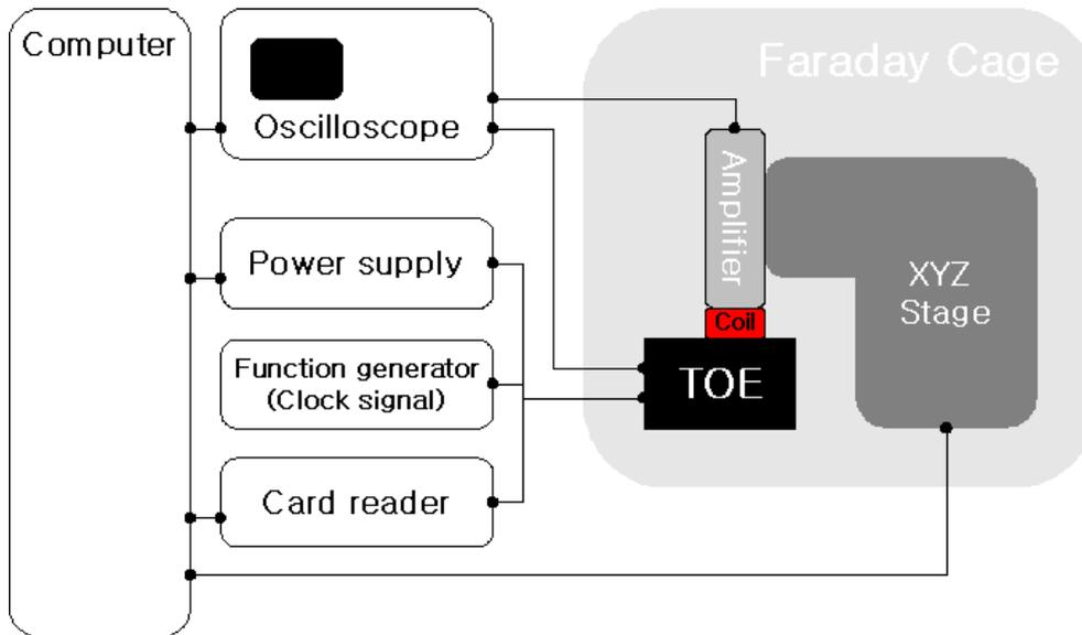
Figure 68: Schematic representation of the set-up (contact) for measuring electro magnetic side channels.
