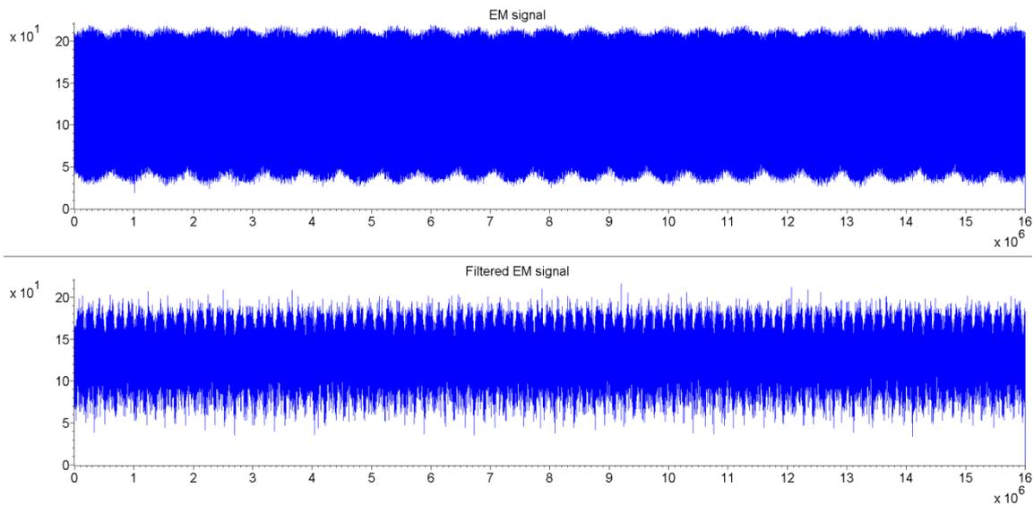
Figure 44: Raw and filtered power trace of the GET\_RAW command.
