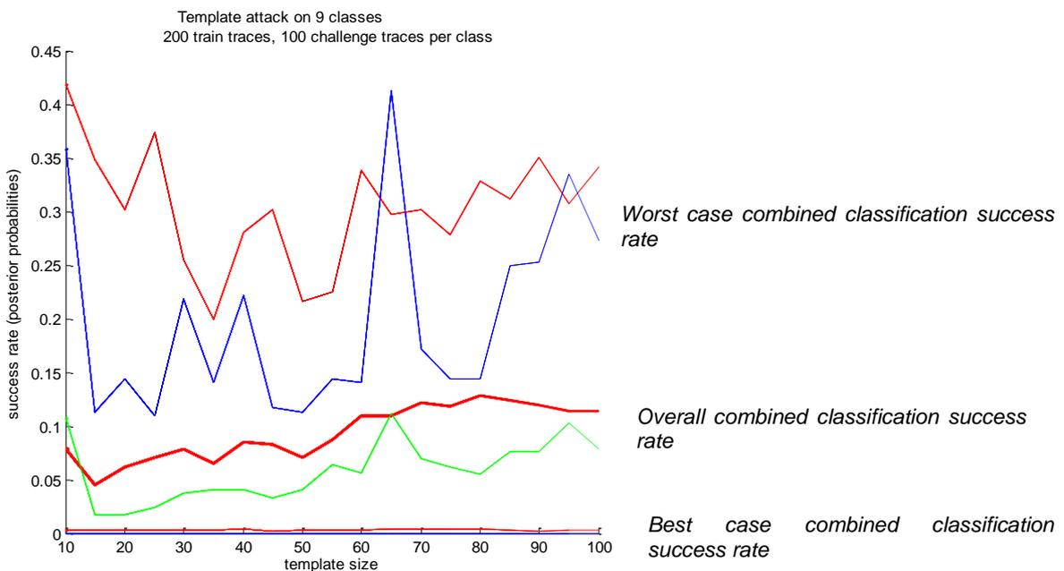
Figure 70: An example of template attack results with optional overall, worst case, and best case combined classification success rates.
