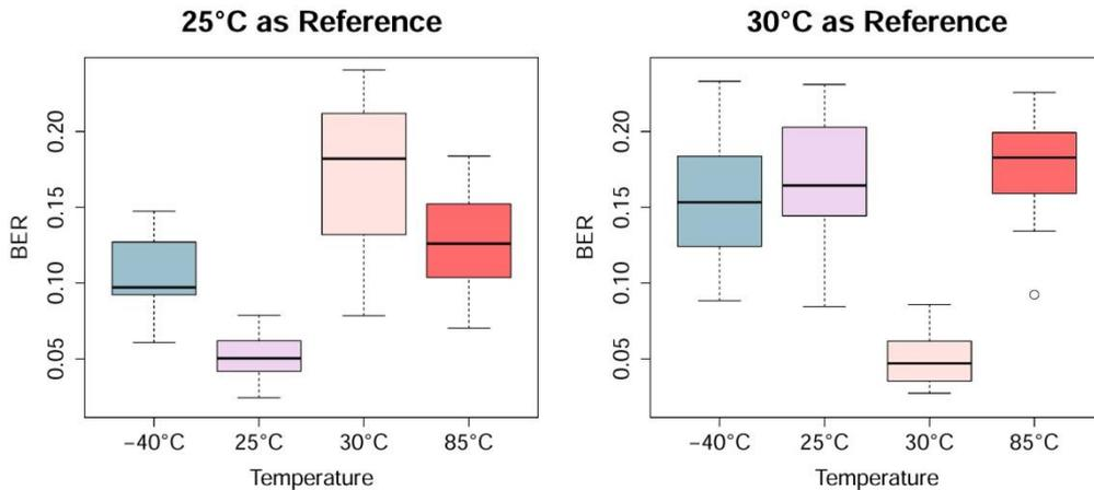
Figure 21: BER of all boards to reference response at 25°C resp. 30°C
