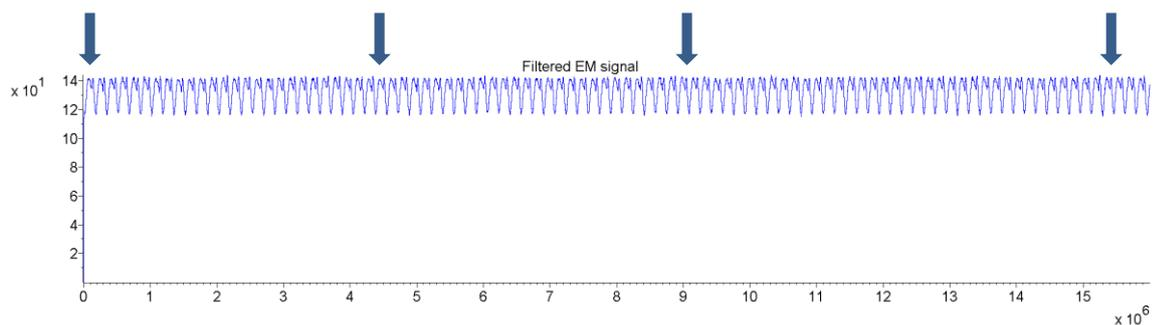
Figure 45: Filtered EM trace with applied time filtering.
