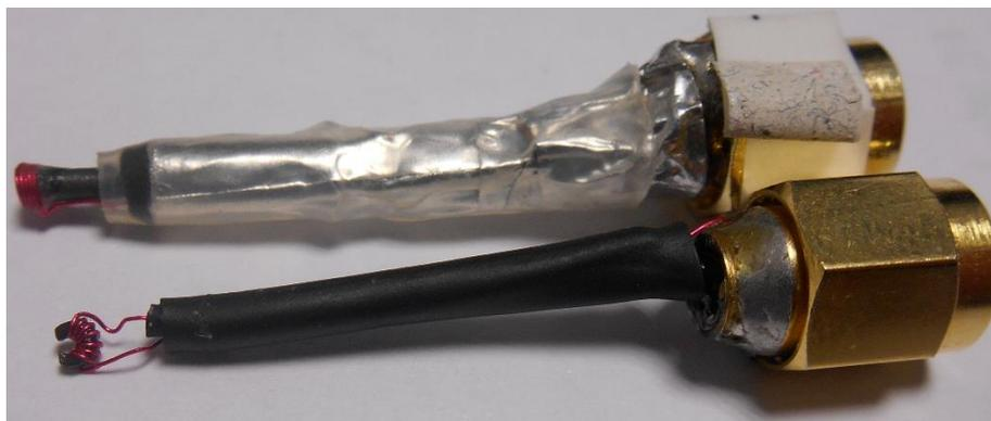
Figure 60: EMFI probes used for characterization
