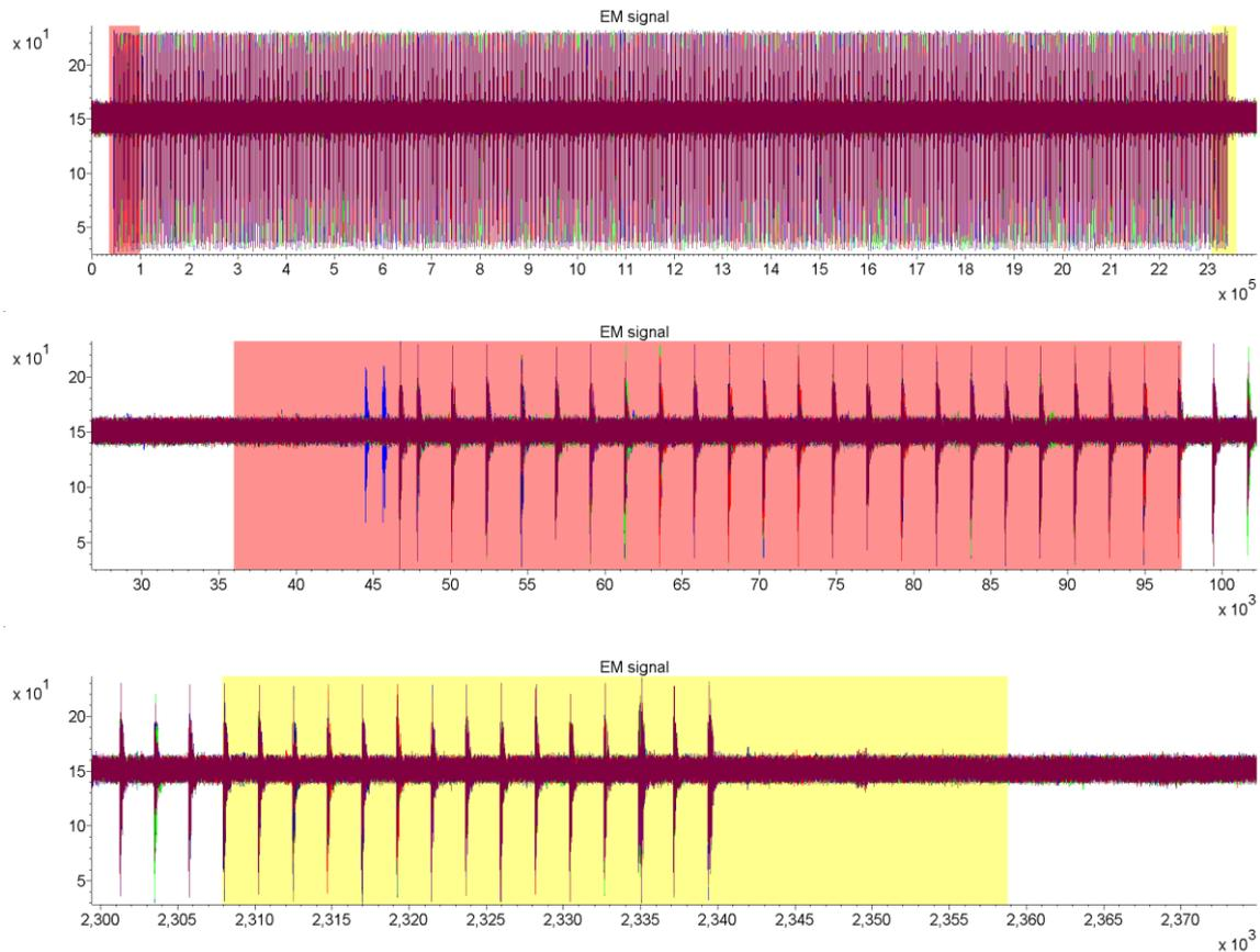
Figure 26: Ten overlaying traces (top) and the zoomed in views of the intervals marked by red and yellow. No additional alignment was necessary.
