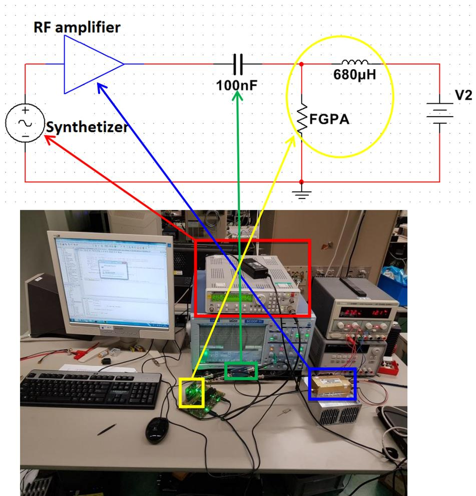
Figure 54: Diagram of the final set-up
