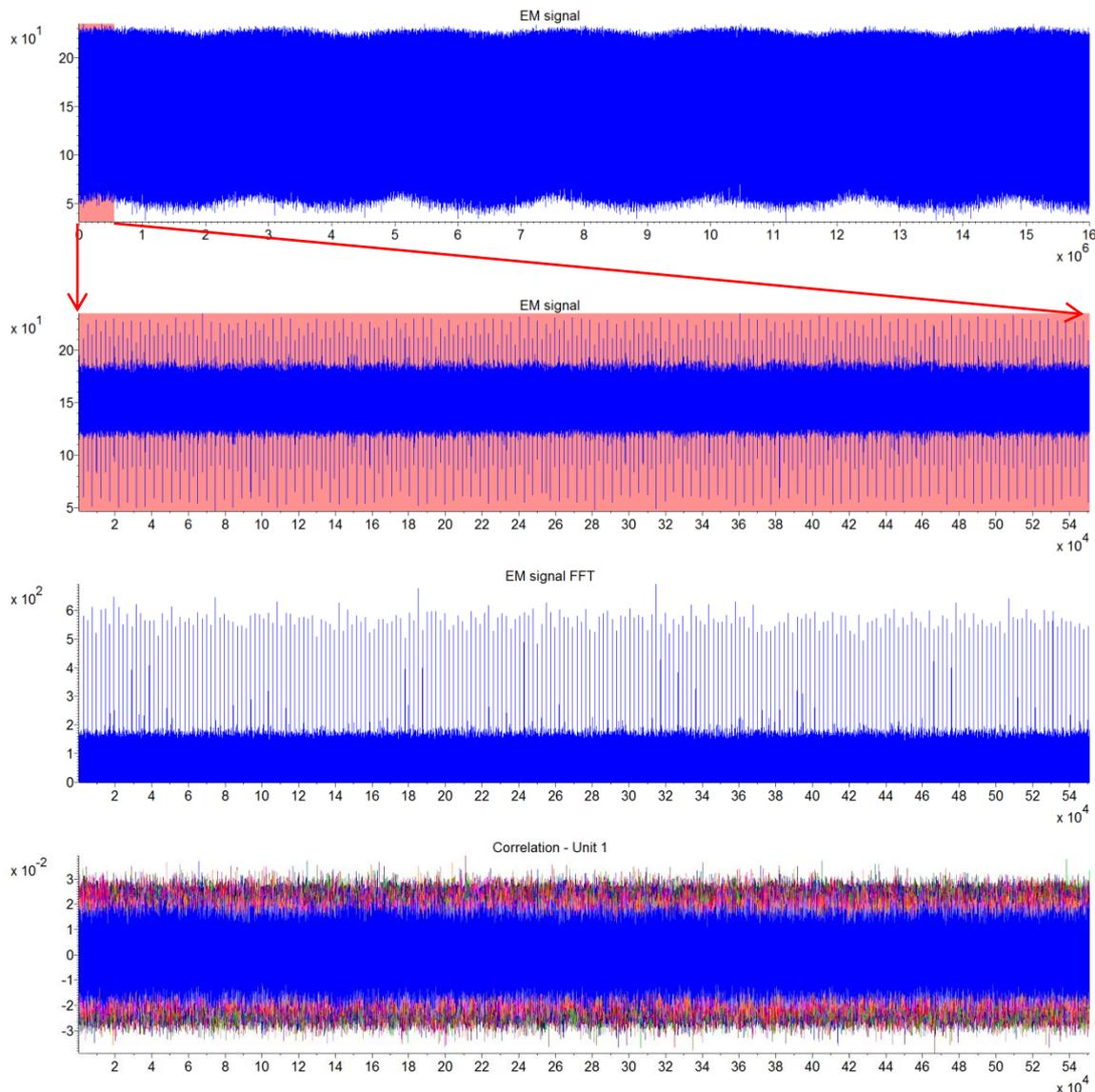
Figure 52: One of the measured EM signals (1<sup>st</sup>) with a zoomed-in view (2<sup>nd</sup>) of the interval used for one of the FFTs. The resulting FFT trace (3<sup>rd</sup>) and the correlation result (4<sup>th</sup>).
