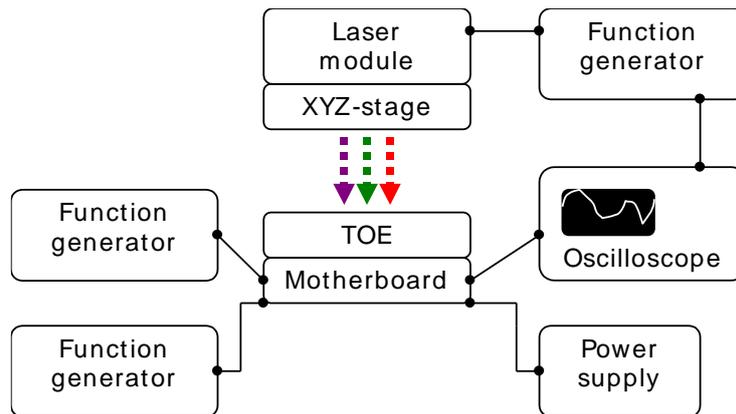
Figure 66: Schematic representation of the LM4, LM6 and LM8 set-ups (contact mode).
