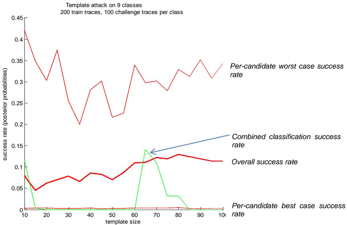
Figure 69: An example of template attack results.
