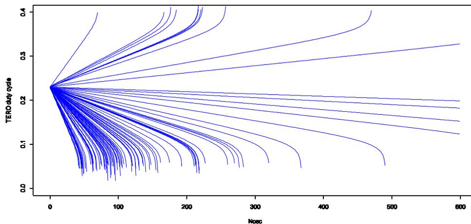
Figure 12: TERO output duty cycle evolution with process variations on  $V_{tk}$
