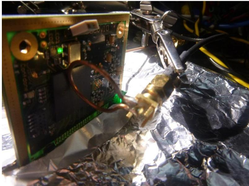
Figure 35: Picture of the TOE and the final coil position.
