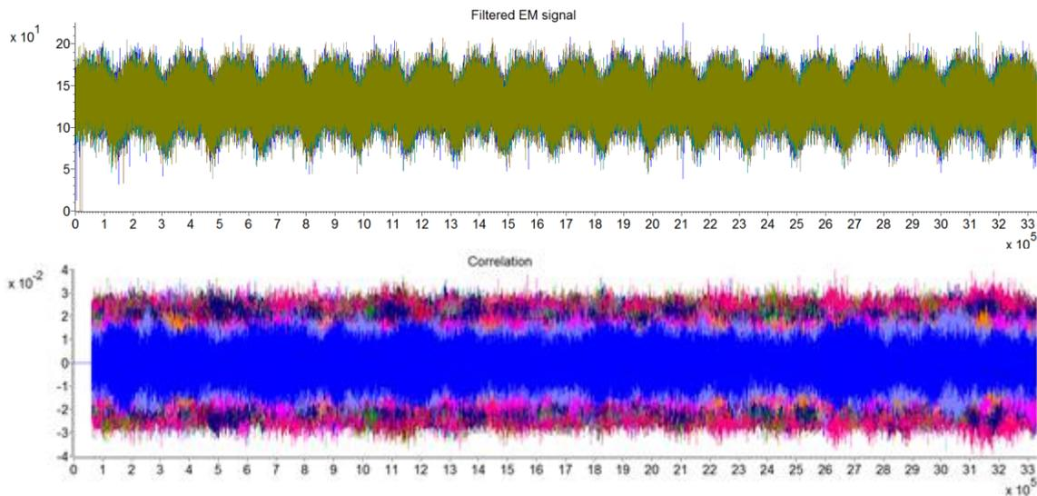
Figure 42: Correlation result for all 256 values of the counter for the alignment in Figure 41.
