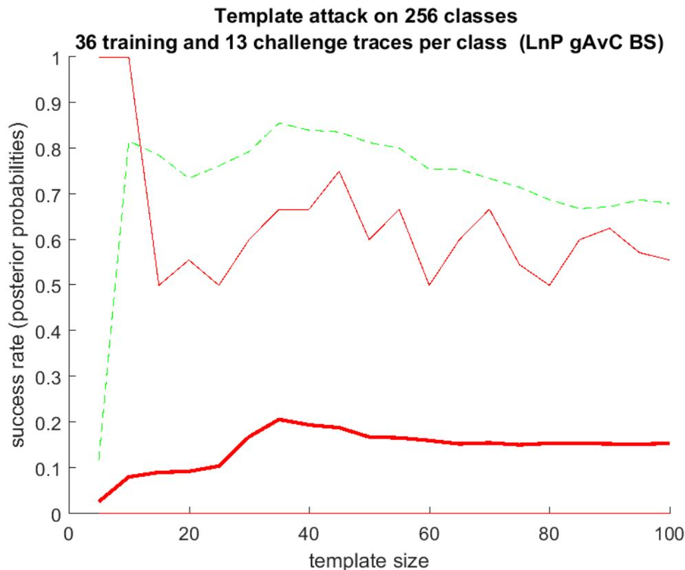
Figure 34: Success rate of the template attack on EM traces, on 256 byte values on the second generated byte as a function of the template size (minimum distance between points of interest equals two and a single covariance matrix was used).
