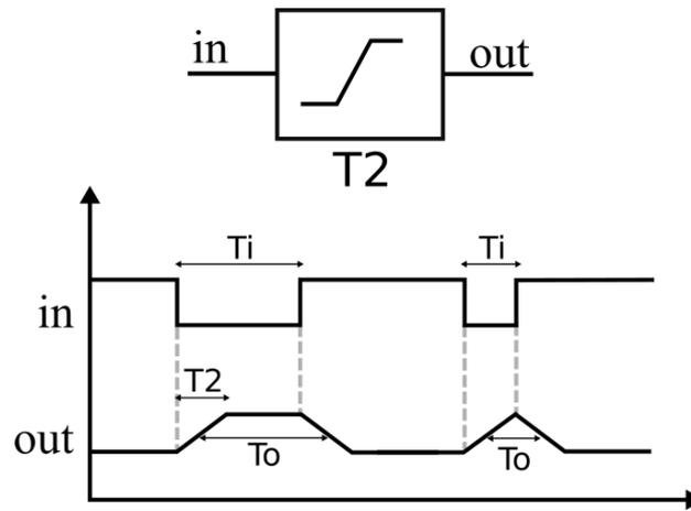
Figure 9: Slope limiter effect
