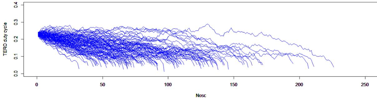
Figure 13: TERO output duty cycle evolution with jitter noise
