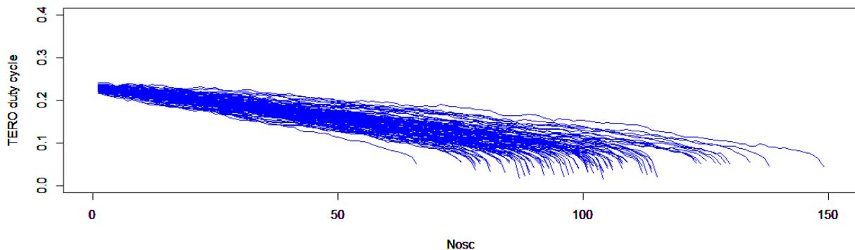
Figure 14: TERO output duty cycle evolution with voltage variation
