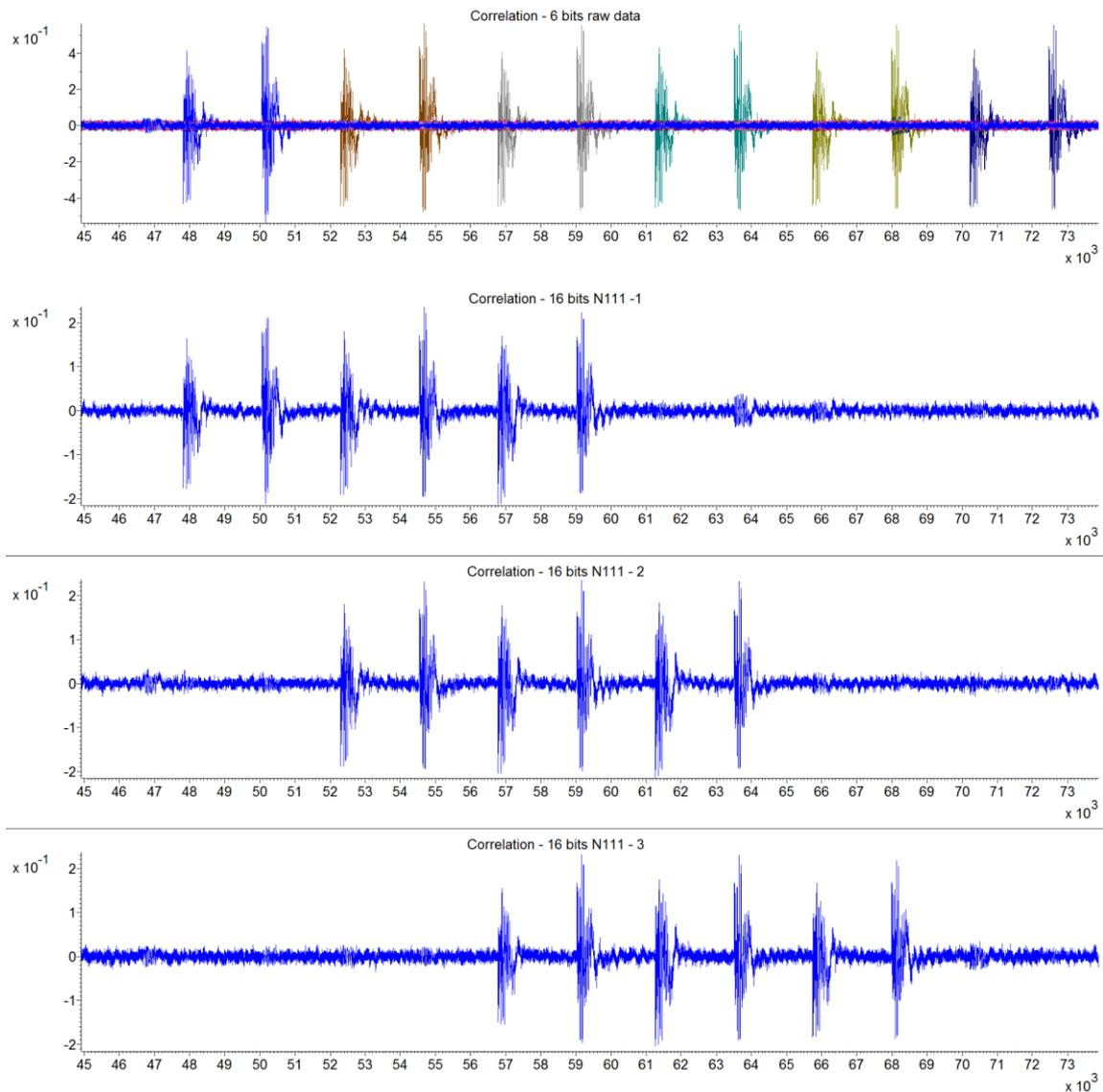
Figure 28: The trace in the top shows correlation results of the first 6 bits of the raw random data. The three traces in the bottom show the correlation results of the first three bits of the data used to calculate  $N_{111}$ .
