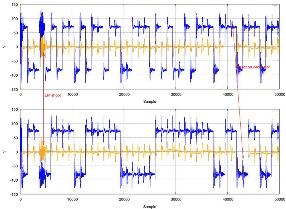
Figure 63: PE stuck at 11. Same color code as figure above. The upper graph represents the PE output and the bottom graph is the decimator output.
