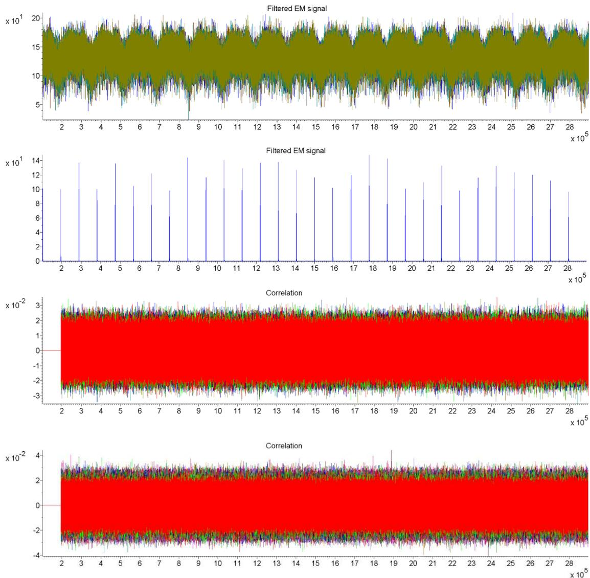
Figure 49: The investigated part of the trace can be seen in the top. The second graph shows a converted trace. The lower both graphs show correlation traces for the first eight bytes (third graph) and for the first 64 bits (bottom graph).
