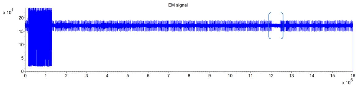
Figure 33: An example trace of the third measured set with configuration 5. The brackets mark a gap in the trace, which appears 13 times in the first 50 traces.
