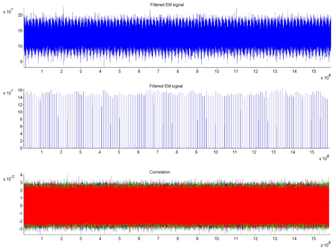
Figure 43: In the top a filtered EM trace. In the middle the corresponding converted trace in the frequency domain. In the bottom the correlation traces for the first eight byte-values of the counter.
