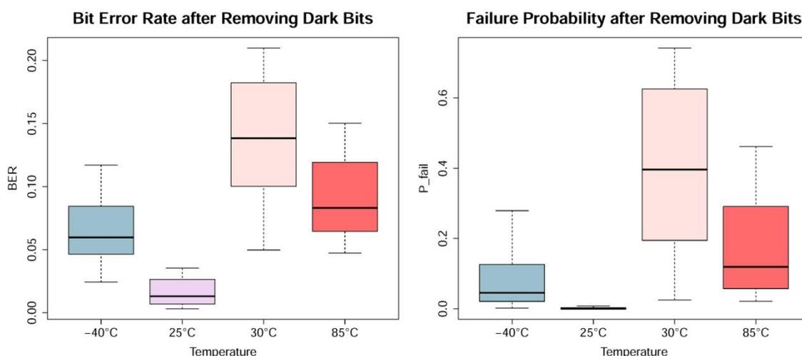
Figure 23: BER and  $P_{\text{fail}}$  of all daughter boards when removing the same dark bits
