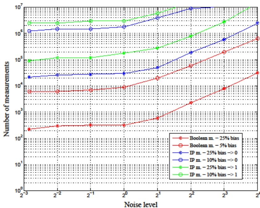
Figure 58: Univariate CPA attacks against AES S-box protected by 1st-order Boolean and IP masking scheme
