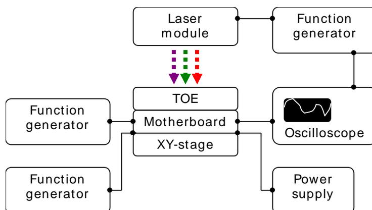
Figure 65: Schematic representation of the LM1, LM3, LM5 and LM7 set-ups (contact mode).
