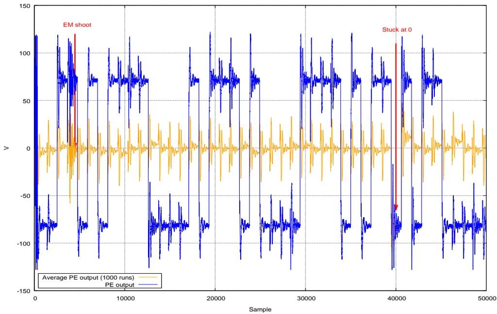
Figure 62: PE stuck at 0 on one bit (blue curves = 1 run, orange curves = average on 1,000 traces)
